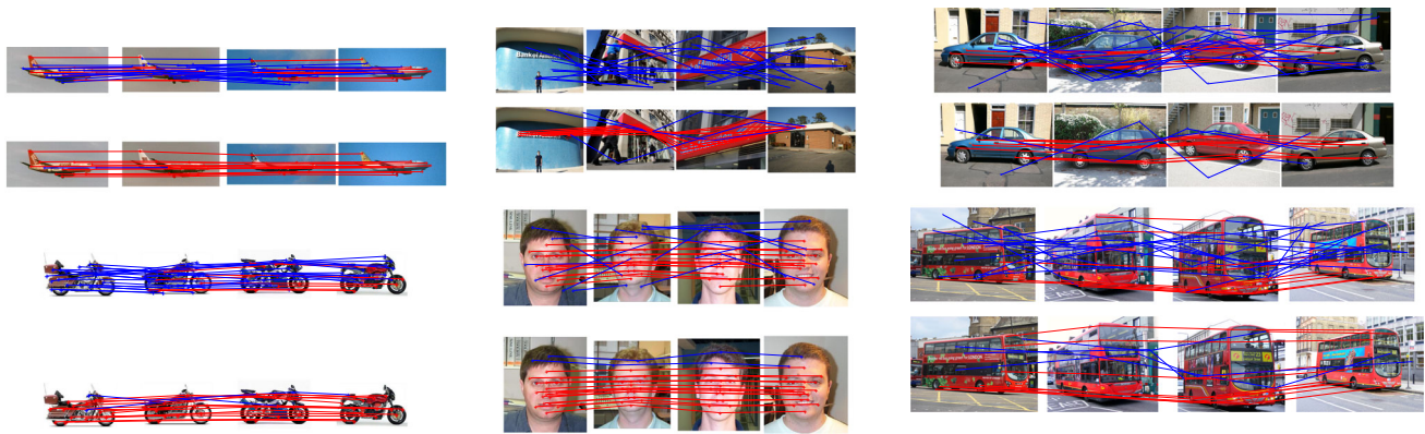
Fig. 3 Example feature correspondences among 4 images for different image sets. For every pair top is from DD (Torresani et al. 2008), and bottom is from our method. Red lines represent identified ground truth correspondences, and blue lines are for false ones (Color figure online)
